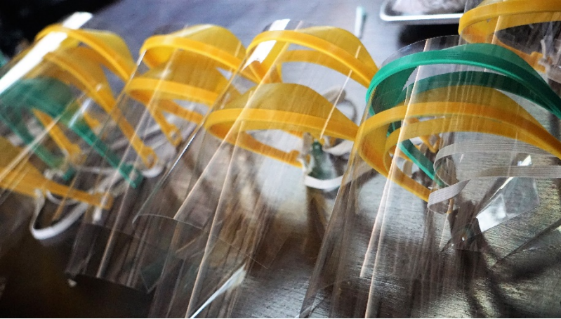
A batch of face shields created with the 3D printer. On average, it takes 2 hours to prepare one such shield. ELVIS RIVERA
