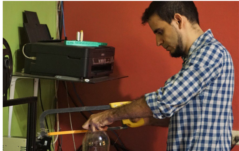
Elvis is cutting PET (polyethylene terephthalate) soda bottles for the face shields transparent component. ELVIS RIVERA
